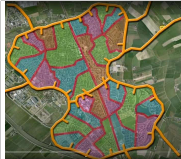
Figure 33: Plan of Houten showing 31 residential areas (red borders) which cars can only enter from the ring road (orange line). Cars cannot cross the red borders
