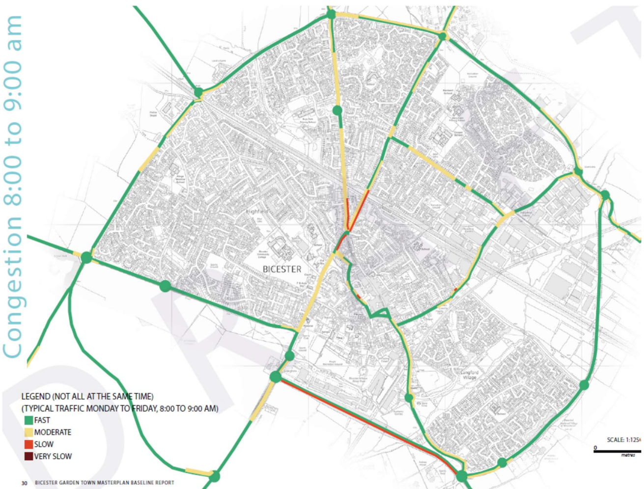
Figure 16 Bicester map showing typical morning (8am -9am) traffic congestion. The worst congestion (excluding the ring road) is on the Central Corridor particularly at the approach to the Buckingham Rd/Banbury Rd roundabout (source Garden Town Master Plan Baseline Report).
